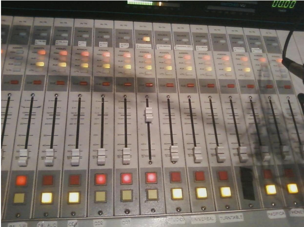
*On-air Studio Audio Board: Setup shown during a successful typical single-channel remote live broadcast, showing the B-PRODUCTION channel used, with the source A/B selector set to 'B'. There may be more enabled channels shown than may be necessary at any given time, depending on the current situation with the on-air programmer.*
